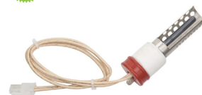
Model ID: BN6612 Voltage: 120 V Cold Resistance: 18-40Ω @25°C Temperature Increase Time: 17Sec reach 1100 °C
