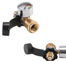
Model ID: BN7702 Inlet Connection: POL (0.880"-14NGO-LH Male) Outlet Connection: 1.312"-5ACME Male & 0.880"-14NGO-LH Female
