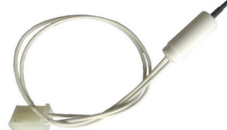
Model ID: BN6611 Voltage: 120 V Cold Resistance: 18-40Ω @25°C Temperature Increase Time: 17Sec reach 1100 °C
