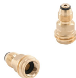
Model ID: BN7706 Inlet Connection: POL (0.880"-14NGO-LH Male) Outlet Connection: 1.312"-5ACME Male & 0.880"-14NGO-LH Female
