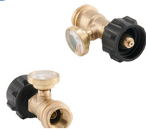
Model ID: BN7701 Inlet Connection: QCC (1.312"-5ACME) Outlet Connection: 1.312"-5ACME Male & 0.880"-14NGO-LH Female
