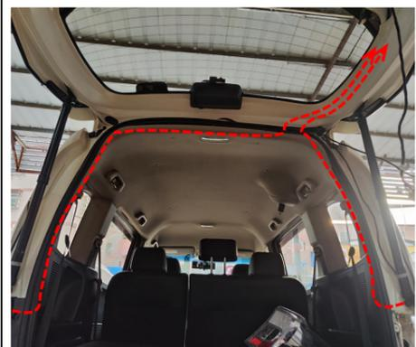
15. Route the strut wiring harnesses.
