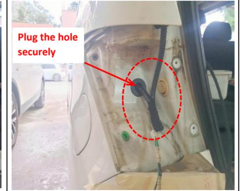
14. Wrap the wiring harness with electric tape and pay attention to avoid pulling it. Plug the holes on both sides securely.
