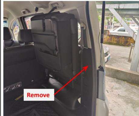
3. Remove the trim panel on the right side of the trunk to allow wiring harnesses to pass through.
