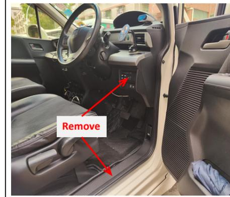
1. Remove the front right side door sill panel and switch panel.
