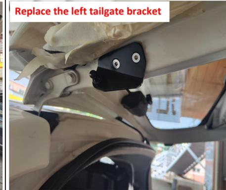
7. Replace the left tailgate bracket with the ball stud near to the hinge.
