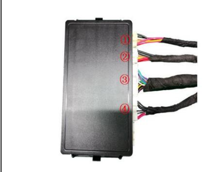
35. Insert the strut wiring harnesses ①②, lock signal harness ③, and power harness ④ into the ECU in sequence.
