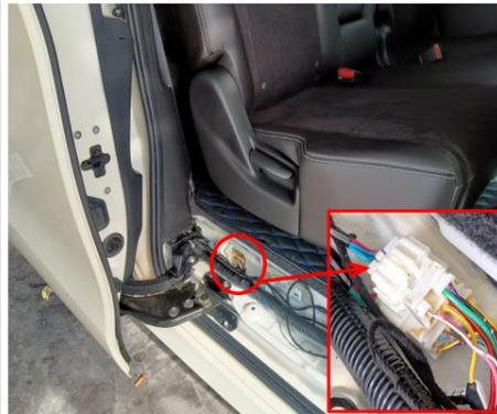
28. Connect the power harness to the indicated signal plugs at the rear right side door (the plug on the top).
