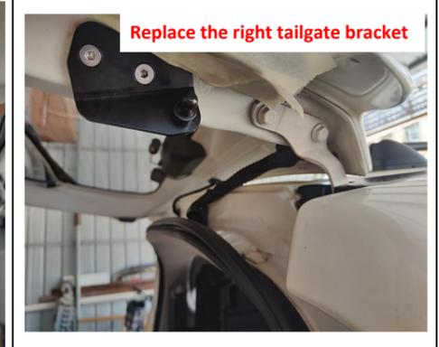
8. Replace the right tailgate bracket with the ball stud near to the hinge.
