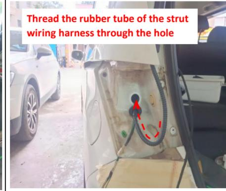
13. Thread the rubber tube of the strut wiring harness through the hole, both sides are the same.
