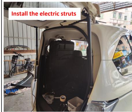
11. Install the electric struts, L on the left, R on the right (the first letter of the strut code), making sure the ends with wiring harnesses are on the vehicle body.
