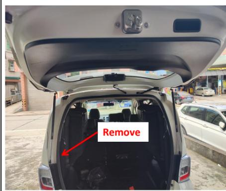
4. Remove the trim panel on the left side of the trunk to allow wiring harnesses to pass through.
