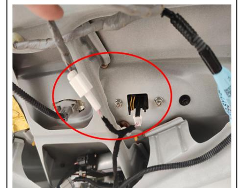
20. Connect the plugs of the lock signal harness to the plugs of the original tailgate switch.
