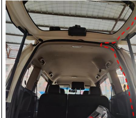
24. Thread the power harness to the tailgate (routing only, no plug or power connection).
