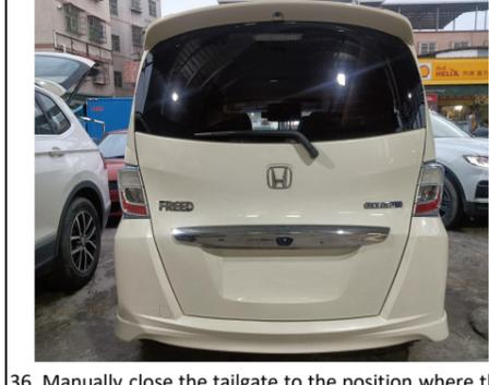
36. Manually close the tailgate to the position where the latch touches the striker and press the added tailgate switch to open and close the tailgate once. The system completes initialization and test each function of the electric tailgate.
