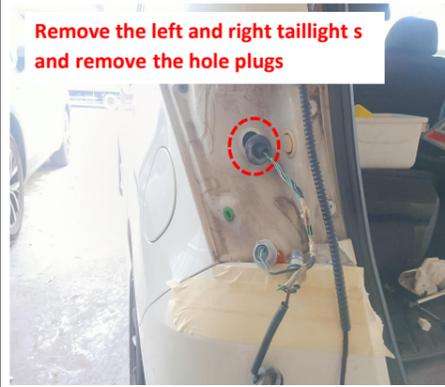
12. Remove the left and right taillight and remove the hole plugs
