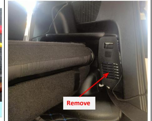
26. Remove the indicated cover panel in the trunk (ground inside).
