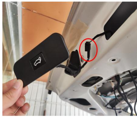
21. Connect the plug of the lock signal harness to the added tailgate switch.
