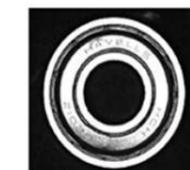
Bearing rust detection, use light source to black rust, white background, convenient software analysis.
